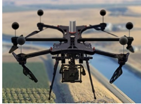
Figure 2.4 SARA Inc.'s PANCAS Airborne DAA System Installed on a sUAS
