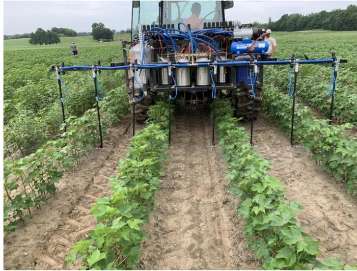
Figure 3.1 Drop-nozzles utilized to evaluate cotton response to currently non-labeled herbicides.
