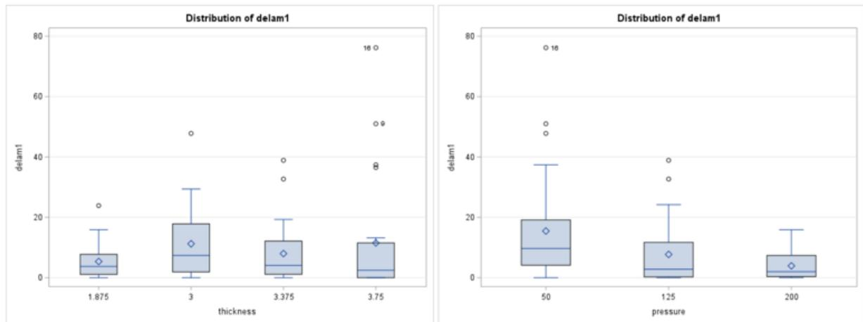
Figure 14 Delamination thickness and pressure box plots
