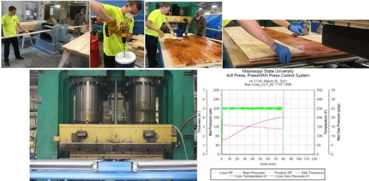
Figure 1 CLT production process
