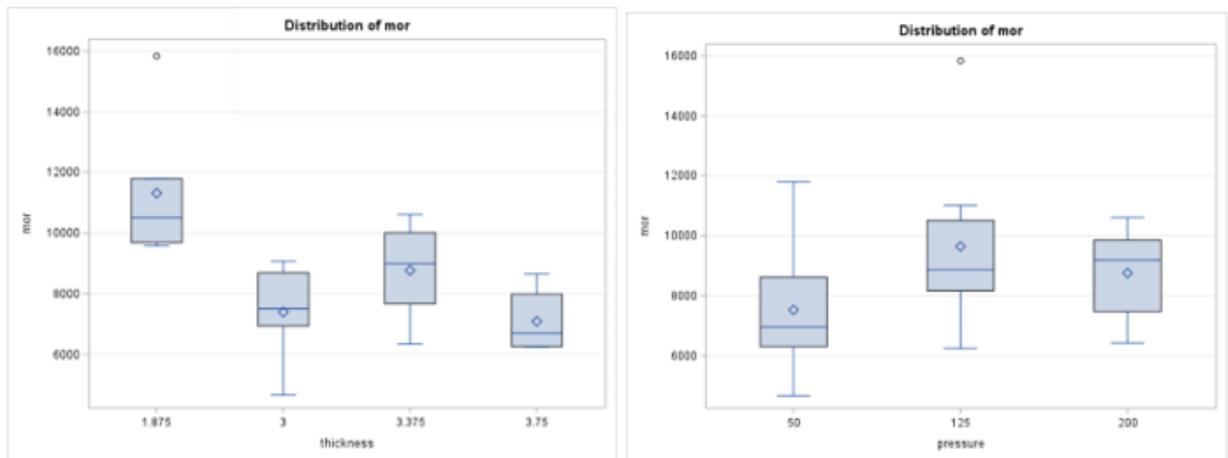
Figure 4 Bending MOR thickness and pressure box plots.
