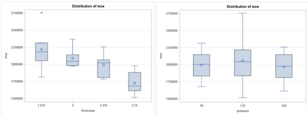
Figure 7 Bending MOE thickness and pressure box plots.
