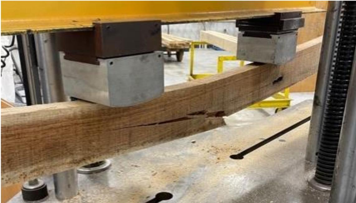
Figure 2.2 Red oak lumber on Tinius Olsen machine before (upper panel) and after failure (lower panel) with the type of failure in static bending cross-grain tension
