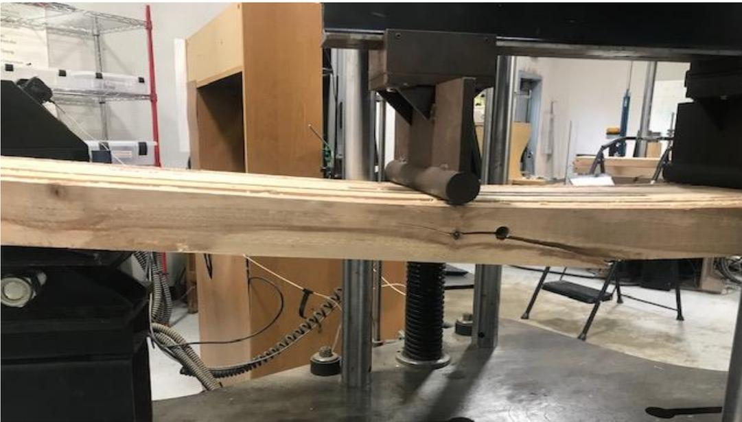
Figure 2.1 Hardwood composite billets on Tinius Olsen machine before (upper panel) and after (lower panel) failure
