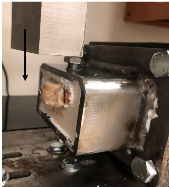
Figure 4 A repaired simulated C3 slab fracture secured in the testing machine.
