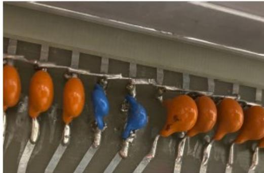
Figure 3.4 An illustration of D0X repair after attaching two new (blue) capacitors to the HV bus.
