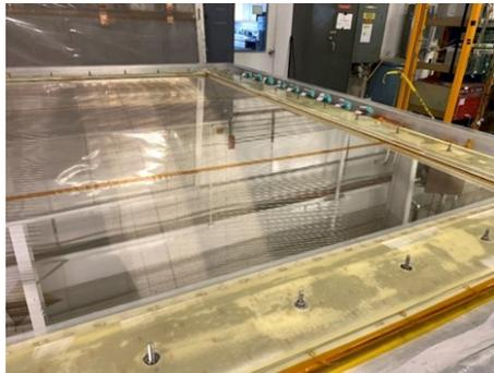
Figure 3.9 D2U sense plane after removing the top cathode plane
