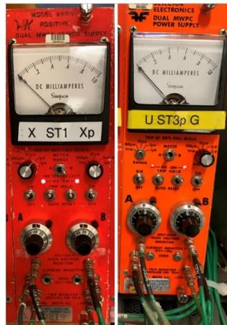
Figure 2.7 Positive (left) and negative (right) HV power supplies used for various drift chambers
