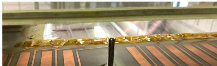
Figure 3.10 Covered resistors with Kapton tape
