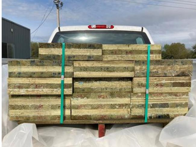
Figure 2.9 Post-treated CLT panels manufactured from southern yellow pine lumber.
