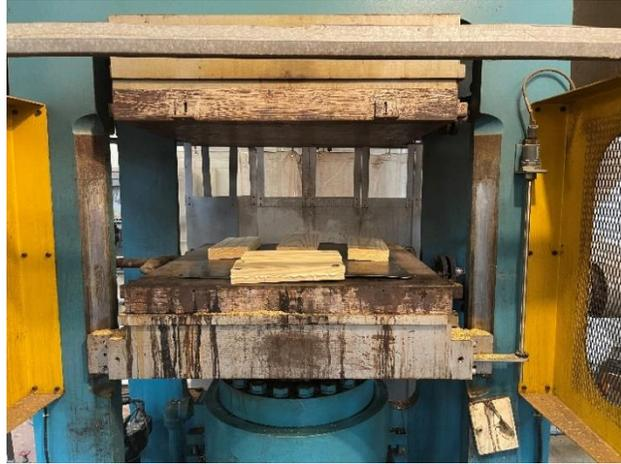
Figure 4.1 Manufacturing of glulam using a laboratory hydraulic press
