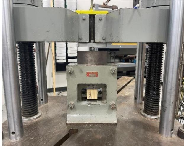
Figure 4.3 Device for the block shear test
